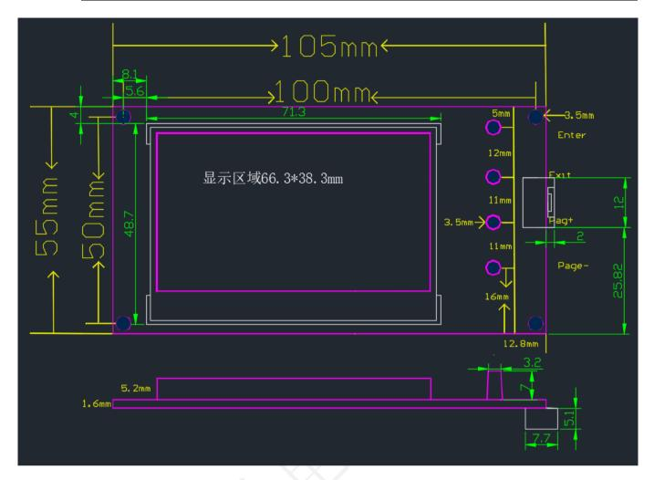
Note: We have two displays: LCD003 and LCD004, LCD003 is regular display and LCD004 is Bluetooth display. The two screens have the same size and hole positioning..
