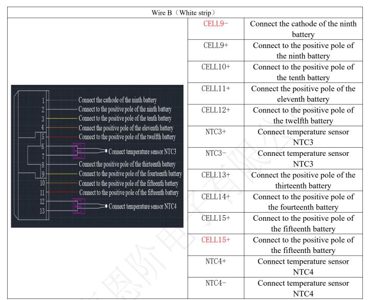
Note: CELL8+ and CELL9- are connected to the positive pole of the 8th cell and the negative pole of the 9th cell to provide cell sampling accuracy; CELL15+ is the B+ terminal of the cell.
