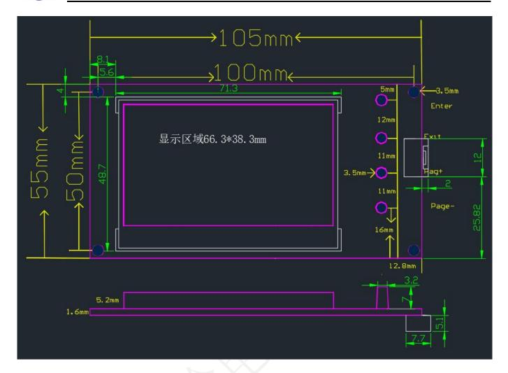
Note: Based on the actual shipment of the display screen, our company has two types of display screens: LCD002 and LCD003. The functions and fixing holes of the two display screens are the same.
